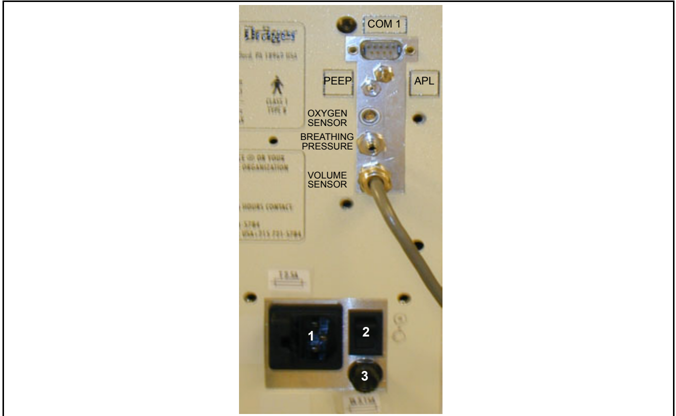
Figure 148. Connector Panel at Back of Machine
